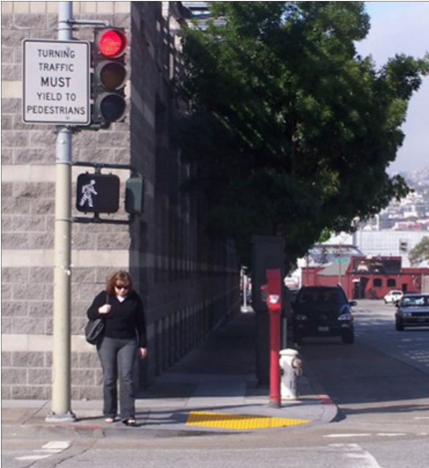
A leading pedestrian interval allows pedestrians to get a head start crossing the street before cars are permitted to go. Source: Federal Highway Administration, United States Department of Transportation
