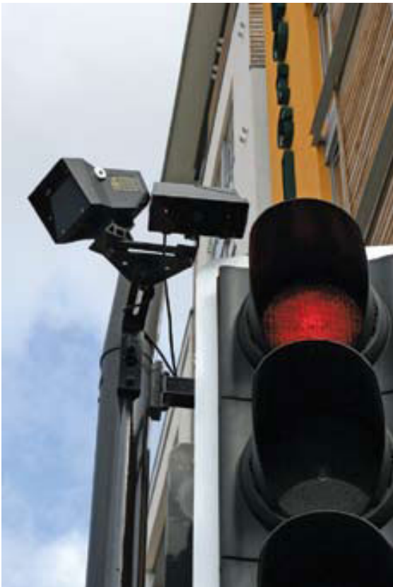
Automated pedestrian sensors for adapting signal timing for pedestrians, Bristol, U.K. Source: Federal Highway Administration, United States Department of Transportation
