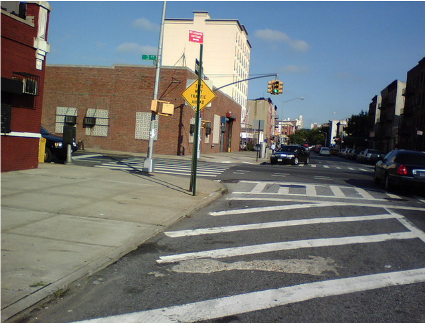
Daylighting at the intersection of Third Avenue at Union Street, Brooklyn, NY. Source: The Consumerist , Flickr
