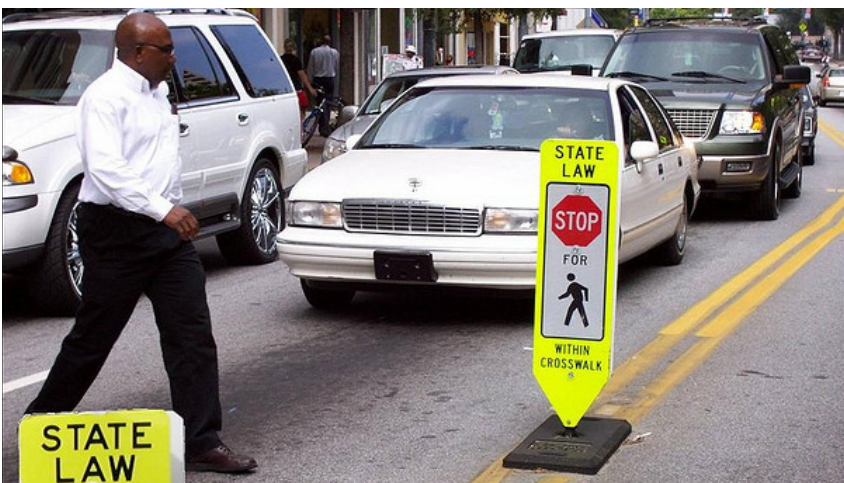
A Stop for Pedestrians in-road sign in Georgia. Source: PEDS.org, Flickr
